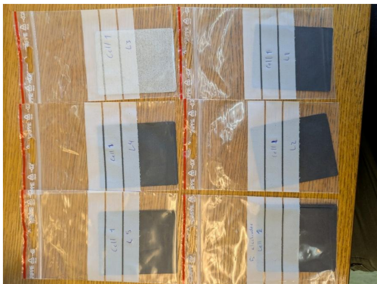
Picture 1. Representative sample of active components (anode, cathode and current collector parts) an equal amount was cut away from each sample in the bags to make up the analysed sample.
